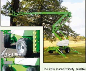
The extra manoeuvrability available from the 4 wheel steer option coupled with the special "Turf Tyres" make the **SD210** ideal for working on sensitive surfaces such as grass.
