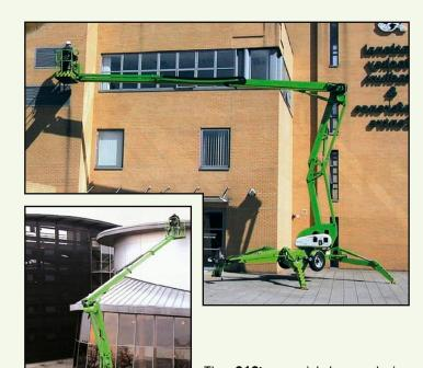
The **210's** special boom design makes it ideal for working near walls or buildings. A single control allows its platform to move vertically while remaining parallel to the job, saving time and improving efficiency.
