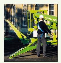
Fully proportional hydraulic outriggers make setting up and levelling quick and easy even on gradients.
