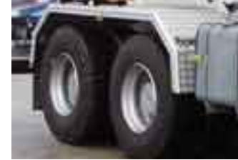
Parafanghi in alluminio Aluminium mudguards
