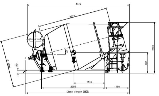
THE CENTER OF GRAVITY DIMENSION ARE REFERRED TO THE MIXER SUB-FRAME.
