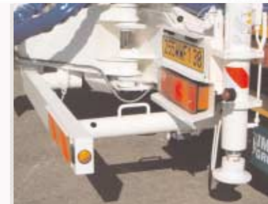
Rear bumper with sensor enabling the conveyor belt movement
