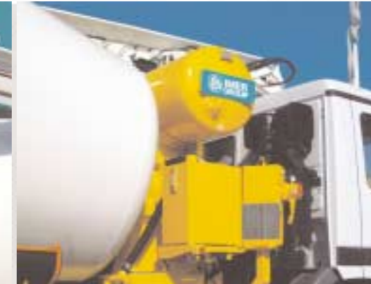
Conveyor belt oil tank hydraulic unit
