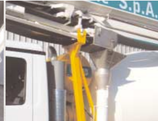
Conveyor belt support: during transport the conveyor belt can be stored on a special support
