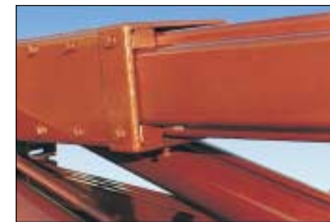
Telescopic jib Rigid and maintenance free, combined with maximum guidance in the jib.
