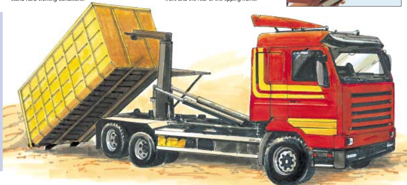
Rollers and Tipping Frame The rollers have a very low build-in height and the special tipping frame is designed to withstand hard working conditions.
