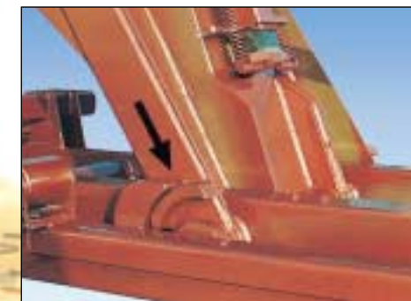
Security Automatic controls to keep the container locked in position during transport.
